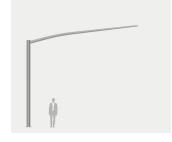
$<sup>^{2)}</sup>$ ) In order to determine the foundation dimensions, please send the catalog cards of the equipment that will be installed on the column and its arrangement. For the values presented in the chart and the arrangement of signaling devices as shown in the diagram below, it is recommended to make a cast foundation with dimensions LxBxH=0,6x0,6x1,6m
